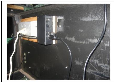
The sockets on the tailgate. I have mounted these in a 'jiffy' box and screwed it to the tailgate
